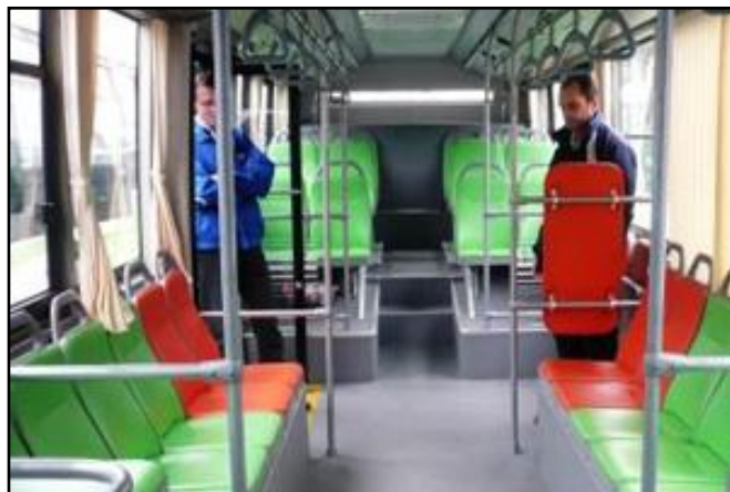
Figure 3.5: Interior of a low entry bus by Volvo
