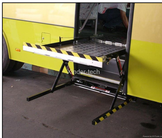
Figure 3.7: Wheel chair lift mechanism in buses
