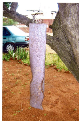
Figure 12 Side-view of the church bell with curved edges resulting from ages of ringing it.
